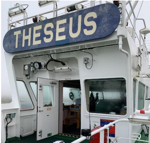
Figure 3 Bad because the wheelhouse is too close and blocking 40% of the sky
