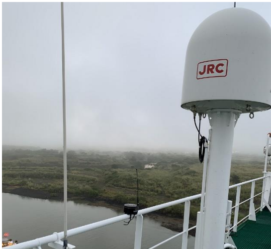
Figure 4 Compromise because antennas block large part of the sky and they might transmit high power
