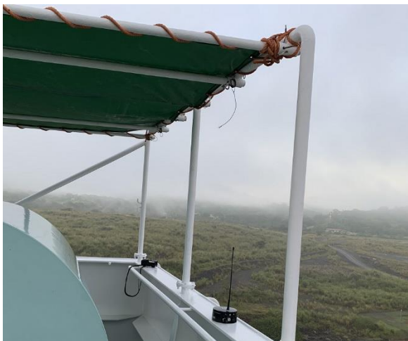
Figure 5 Compromise because pipes are next to and above the CAT PRO
