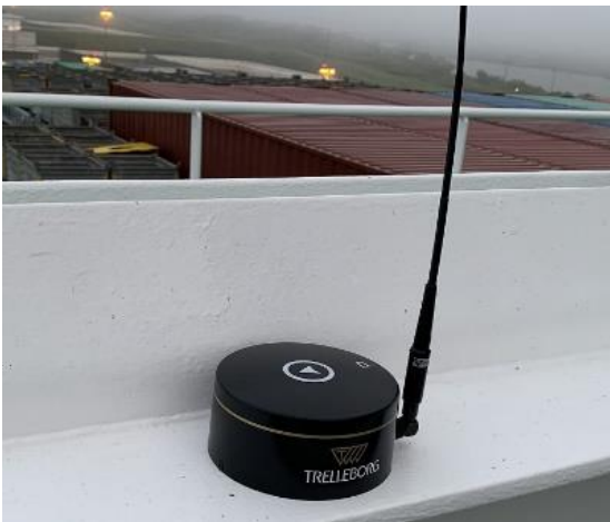
Figure 2 Bad because of the vertical wall next to the unit. A very large part of the sky is blocked and the wall close by will cause multipath
